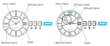
a) Normal position : winding up the mainspring (manual operation)
